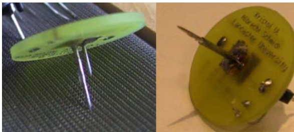
Figure 3. The two connectors. Left: the current two-pin arrangement, right: the prototype with one pin.
