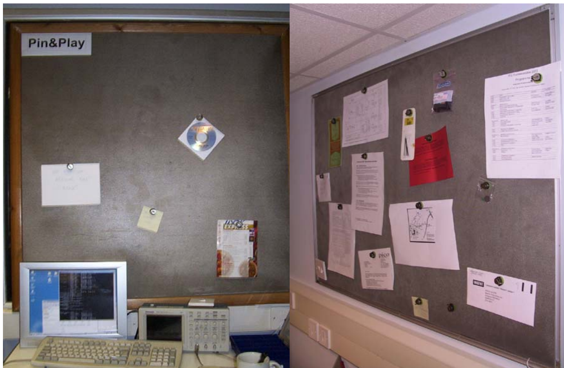
Figure 5. Some of our bigger Pin&Play surfaces. Pins can be moved from one board to another without loss of data, time or calendar, even when the two boards are not connected via a network.
