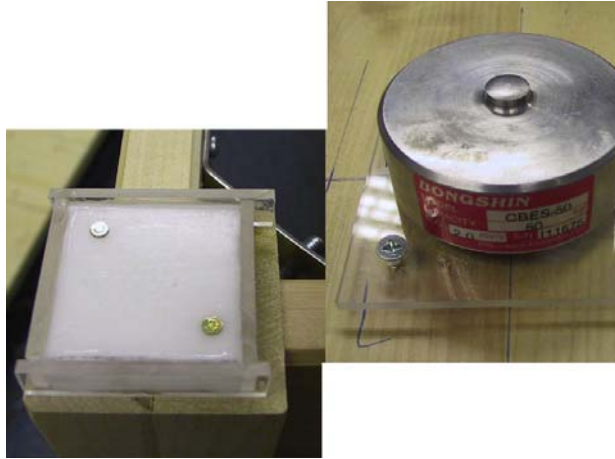
Figure 5. resting point and load cell mounted under the table top of a dining table.
