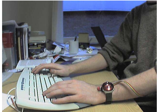
Figure 6. Typical office setting (not glancing at the watch). Connected to the watch is a small board containing the dual-axis ADXL202 accelerometer.
